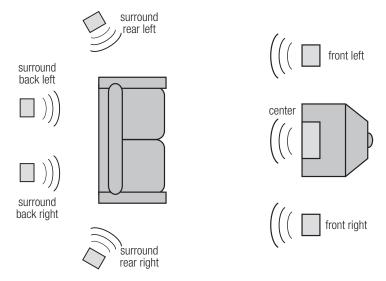
Measure the distance from the listening position to the center speaker and to one of the front speakers. Subtract the center channel distance from the front left or right channel distance. For example, if the front speakers are 12 feet (3.7 m) from the listening position and the center speaker is 10 feet (3.0 m), the difference is 2 feet (0.6 m). For this example the center channel delay is set to 2 milliseconds or ms.
